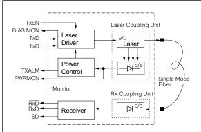
The receiver component converts the optical serial data into PECL compatible electrical data (RD and RDnot). The Signal Detect (SD, active high) shows whether an optical signal is present. If no optical input signal is present the receiver data outputs are switched to static low level (RD=Low, RDnot=high).
