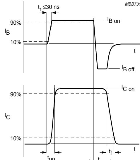
Fig.12 Switching time waveforms with resistive load.
