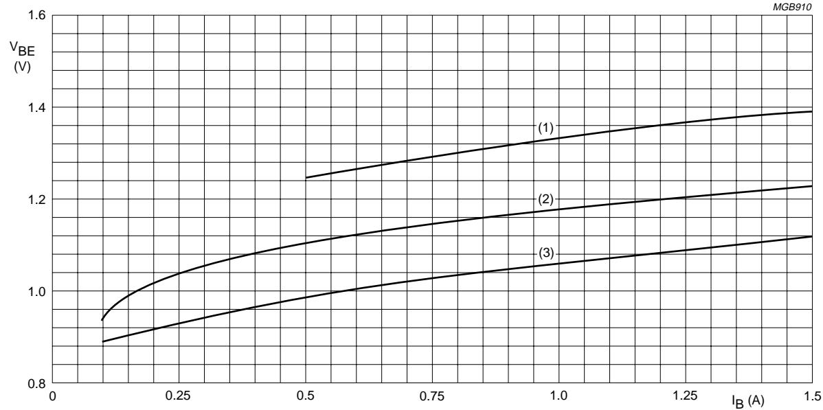
Fig.8 Base-emitter voltage as a function of base current.
