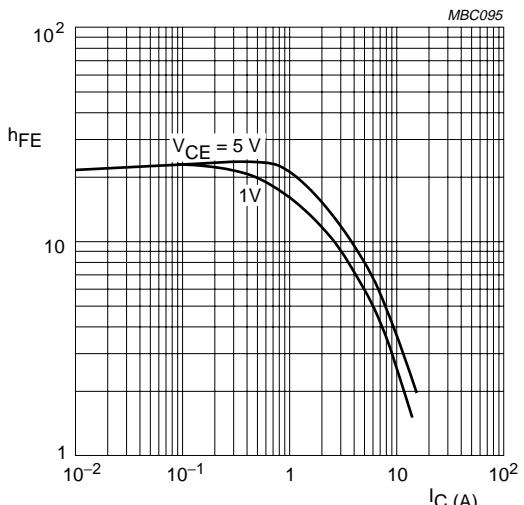
Fig.10 DC current gain; typical values.
