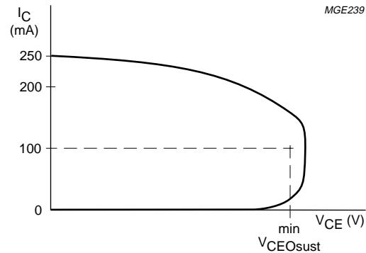
Fig.6 Oscilloscope display for collector-emitter sustaining voltage.
