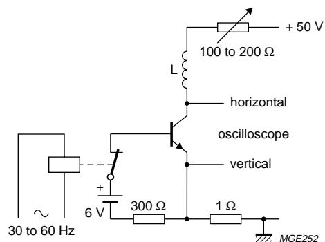
Fig.5 Test circuit for collector-emitter sustaining voltage.
